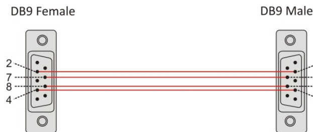
Fig. 26 – Building an extension cable
