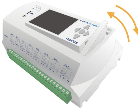
Fig. 10 – Attaching and detaching FieldLogger HMI
