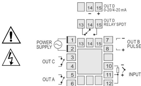
Fig. 1 - Electrical connections of the controller
