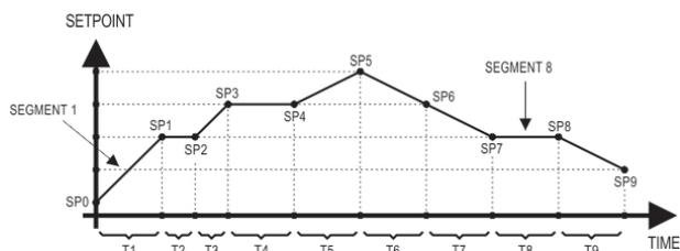
**Fig. 3 - Example of a ramp and level program**
