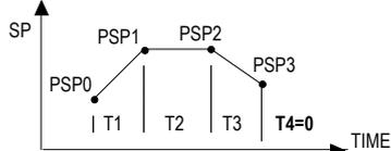
Fig. 4- Example of a program with only 3 segments
